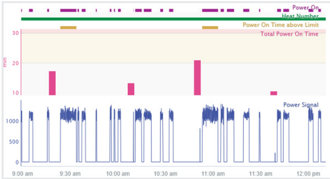
Seeq workbench showing the various heat (or batch number) as well as a calculation of a KPI (Power On Time) over each heat.
