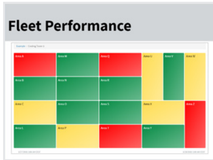
Treemap for a truck fleet highlighting those due for maintenance (in red).
