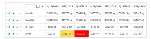
This image shows scorecard summarizing the results of the mass balance. Coloring is used to indicate instances when the mass balance results were not acceptable.
