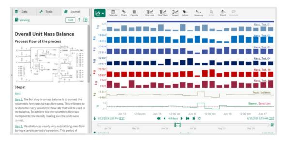
This picture is a screenshot of the workbench analysis, showing the totalized mass for the inlet and outlet streams in the top lanes, and then comparing the difference between these values in the bottom lane.
