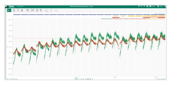
The increase in the calculated filter membrane resistance shows the long-term deterioration of the performance of the membrane, potentially causing increased cycle times, lost yield, or poor product quality.
