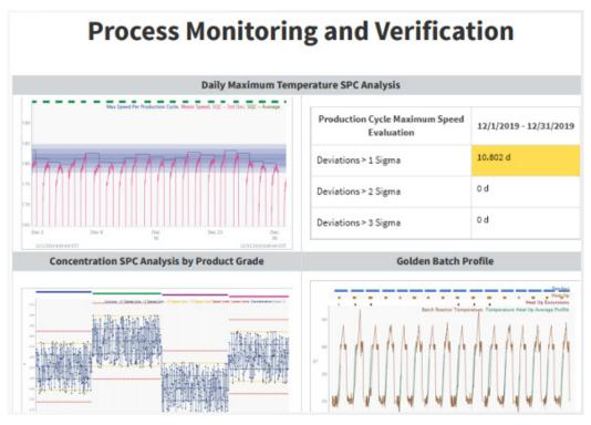
Shown in the picture: A process monitoring report showing SQC limits applied consistently over regular intervals and by product grade, as well as a golden profile. Also shown is a scorecard summarizing deviations.
