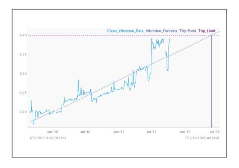
The figure shows a Seeq Analysis with a vibration signal on an induced-draft fan and a predicted vibration forecast.
