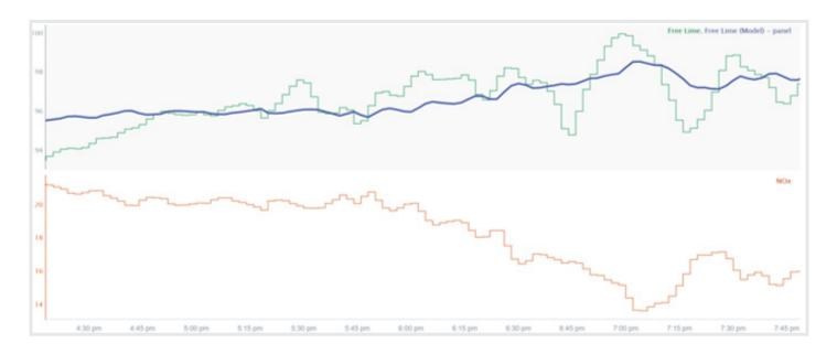
The figure shows an Analysis in Seeq Workbench. The top lane displays the model output overlaid with the actual value of the free lime. The bottom lane is in the NOx value used as the input to the model.
